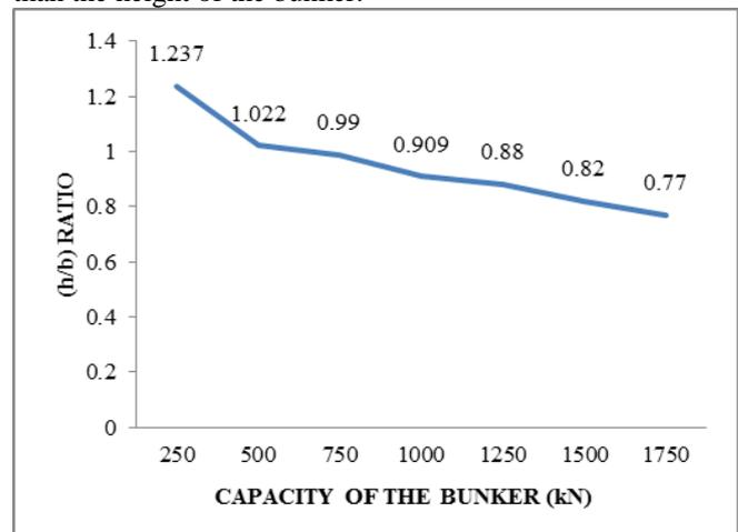
Fig. 6: Variation of (h/b) ratio along the bunker capacity
