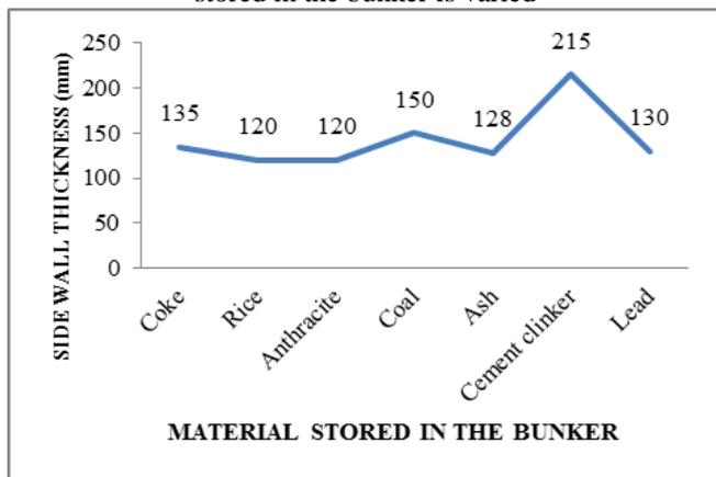
Fig. 7: Variation of side wall thickness for different materials stored in the bunker
