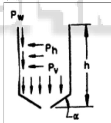
Fig. 2: Pressures acting on the bunker
