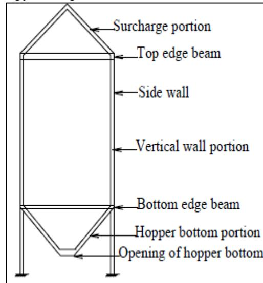
Fig. 1: Typical bunker section
