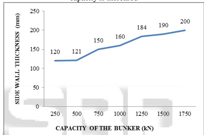
Fig. 5: Variation of side wall thickness along the bunker capacity
