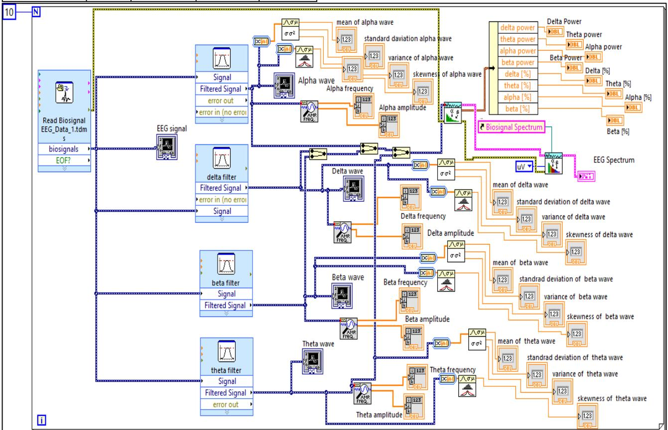
Fig. 8: Block diagram of the feature extraction in lab view
