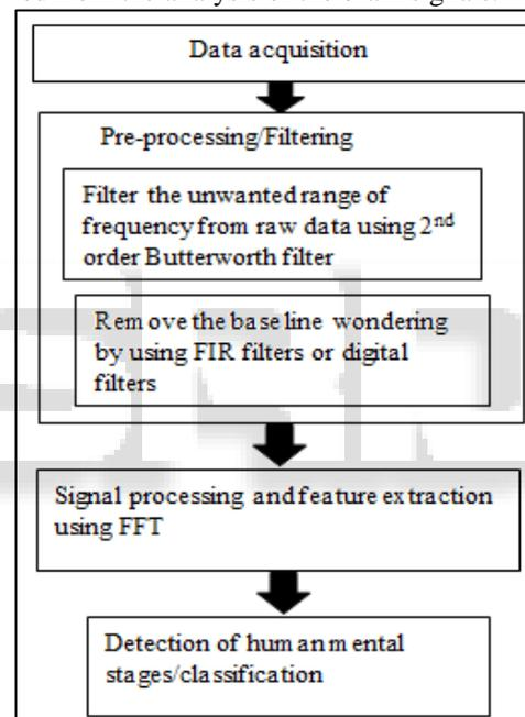
Fig. 2: Structure of complete process of EEG signal
