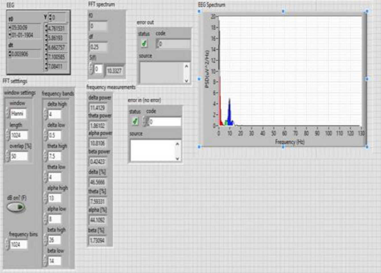
Fig. 7: Front panel of FFT frequency spectrum
