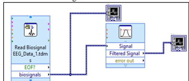
Fig. 5: Filtering of EEG signal with FIR digital filter
