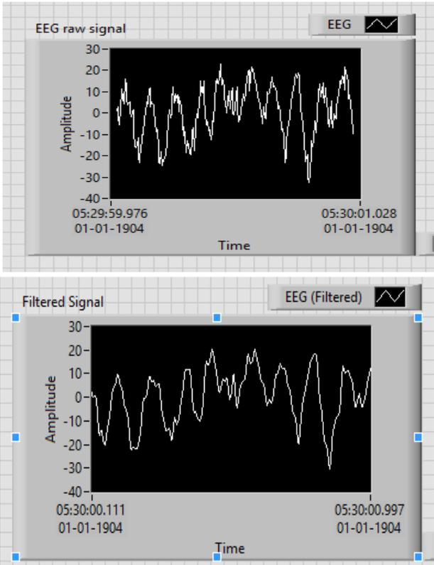
Fig. 6: (1) EEG Raw Signal (2) Filtered Signal
