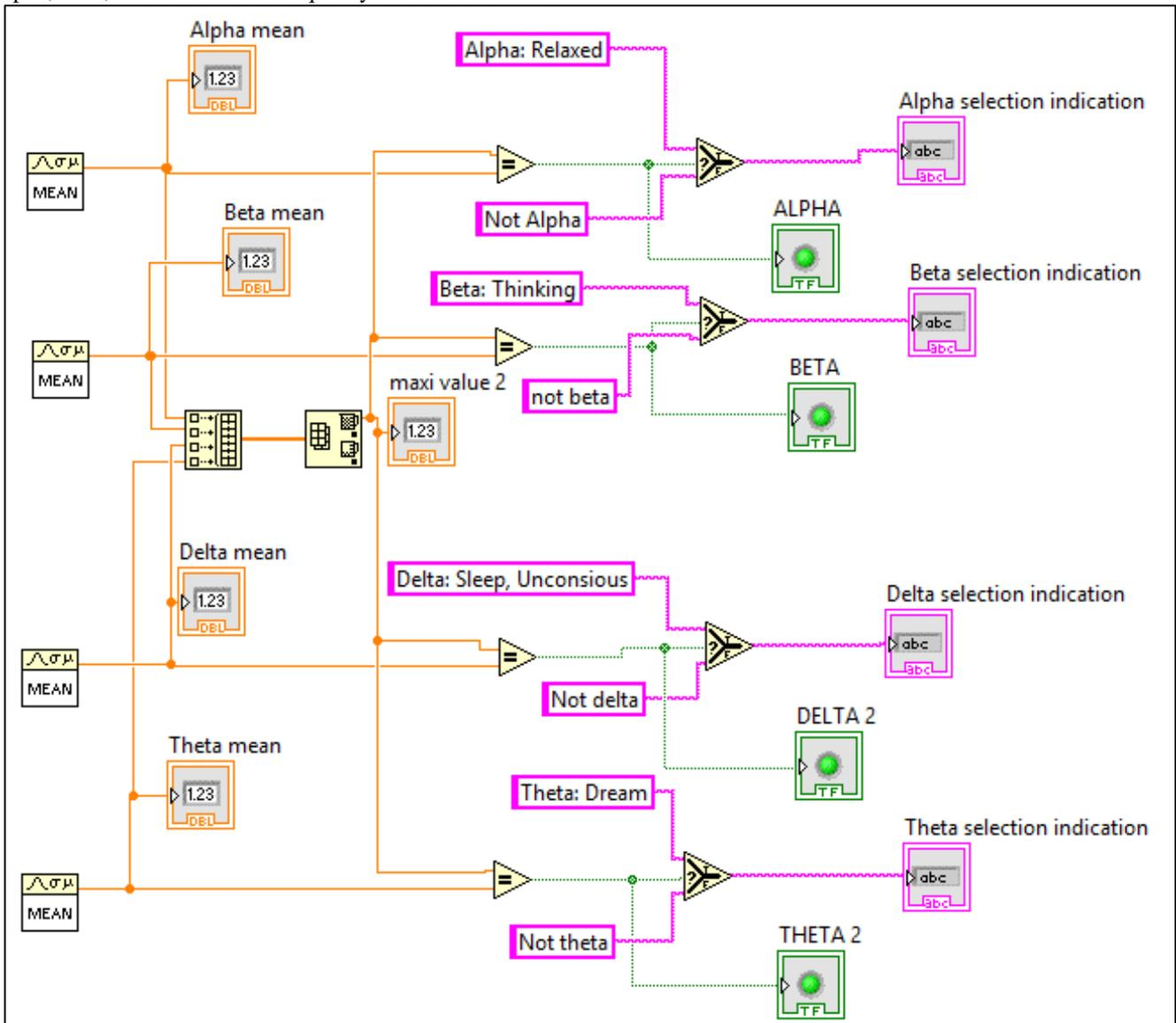
Fig. 10: Labview block diagram of detection of human sleep stages
