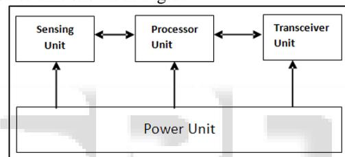
Fig. 1: Components of Wireless Sensor Network
