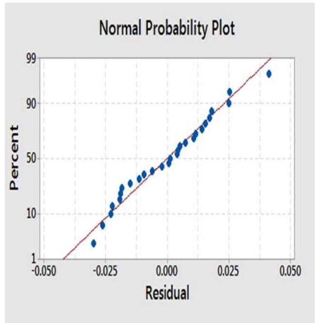
Fig. 4.1: Normal Probability Plot of Residuals for Surface Roughness
