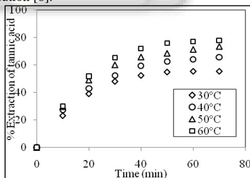
Fig.2. Effect of temperature on extraction of tannic acid [solvent: water, agitation speed: 500rpm and raw material (gm): volume of solvent (ml): 0.3%, diameter of solid: 0.60 ~ 0.85mm].
