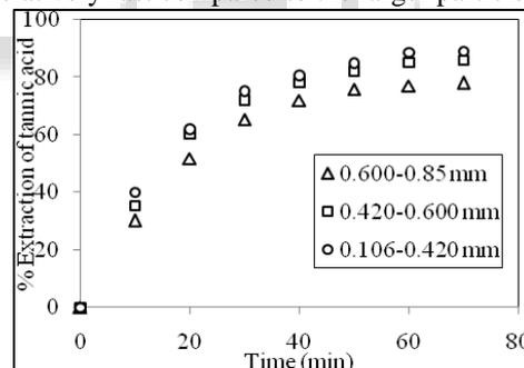
Fig. 4: Effect of diameter of particle on extraction of tannic acid [temperature: 60°C, speed of agitation: 1000 rpm and solid to solvent ratio in percentage: 0.3%]
