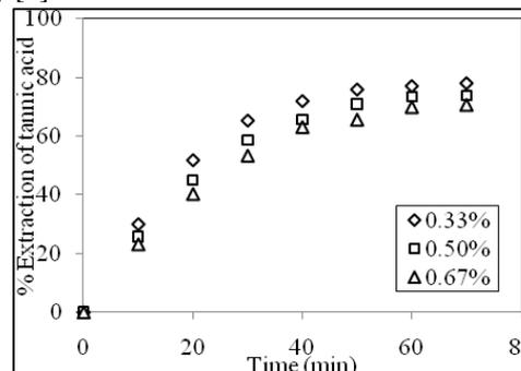
Fig. 3: Effect of solid loading on extraction of tannic acid [solvent: temperature 60°C, speed of agitation: 500 rpm, diameter of solid- 0.60 ~ 0.85mm].
