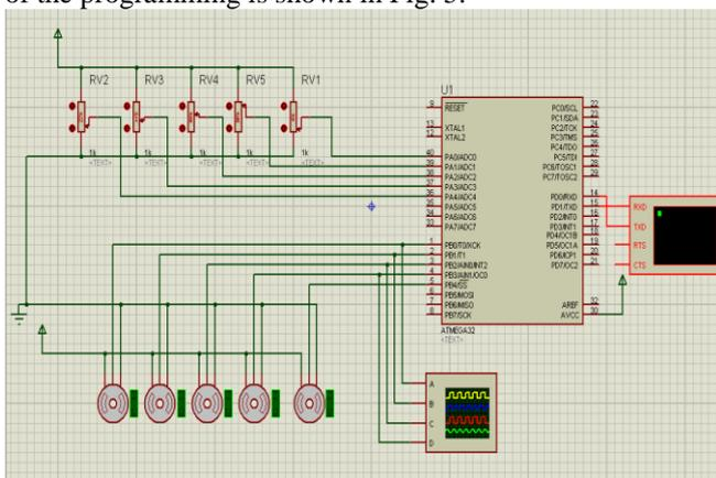
Fig. 4: Simulation Circuit of Servomotor Control using ATmega32
