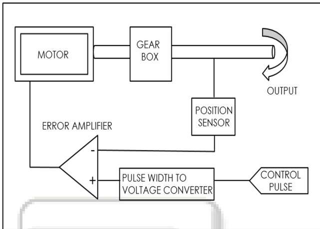
Fig. 3: Internal Construction of Servo
