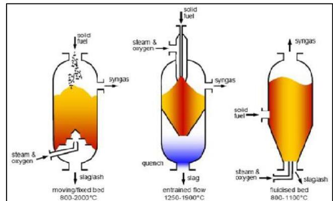
Fig. 1: Types of Gasifier [6]
