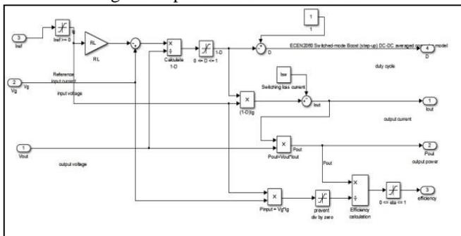
Fig. 7: Simulink model of boost efficiency circuit
