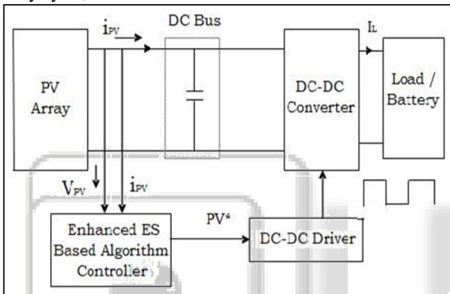
Fig. 1: System Configuration of PV System [19]
