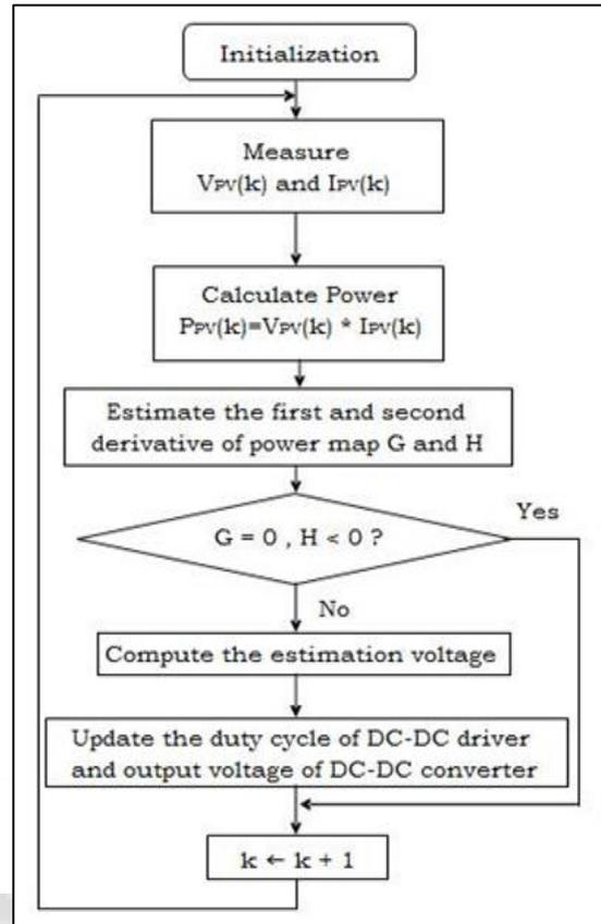
Fig. 2: Flow chart of enhanced extremum seeking MPPT method [19]
