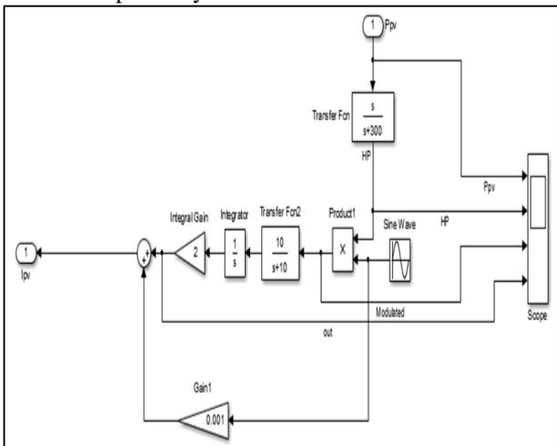
Fig. 3: Shows Esc Mppt simulation block
