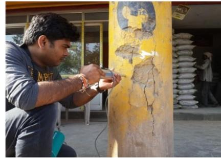
Fig. 1: NDT of damaged structures
