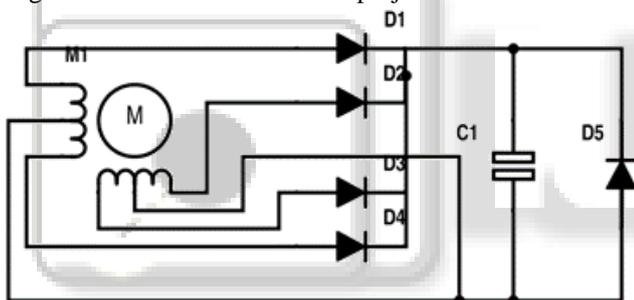
Fig. 2: Circuit Diagram of the Steppermotor
