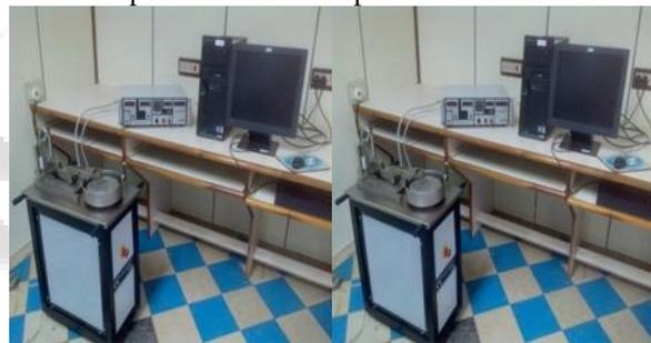
Fig. 4: Pin on disc wear tested specimen.
