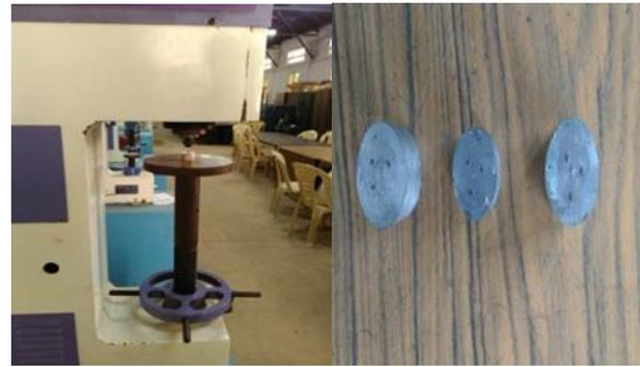
Fig. 3: Brinell hardness tested specimen
