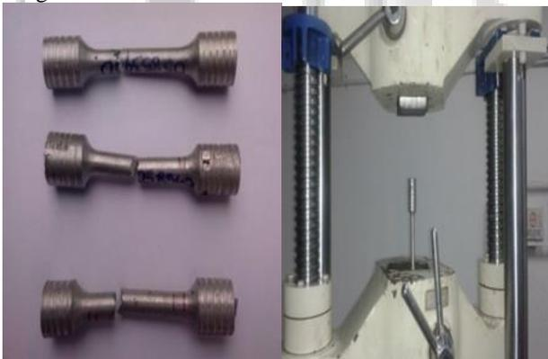
Fig. 2: Tensile test specimen
