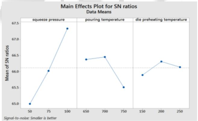
Fig. 5: Response curve for Tensile strength, Hardness, Wear rate
