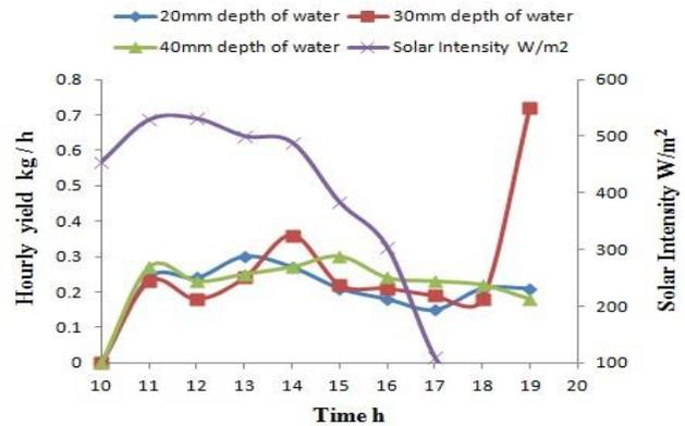
Fig. 3: Hourly yields for different depths of saline water and for the same climatic condition in the modified Still using earth heat
