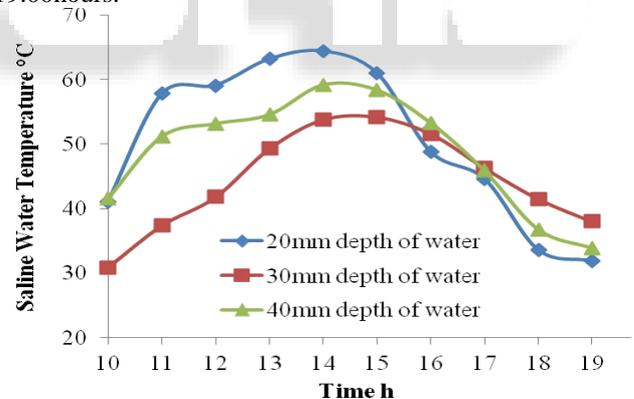
Fig. 4: Saline water temperatures for different depths of saline water and for the same climatic condition in the modified still using earth heat without Energy storage medium
