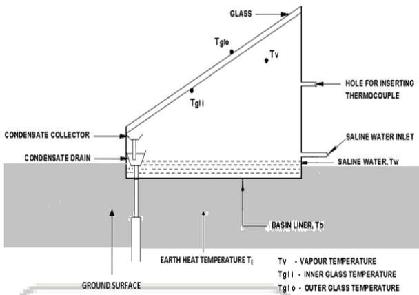
Fig. 1: Sectional view of the solar still
