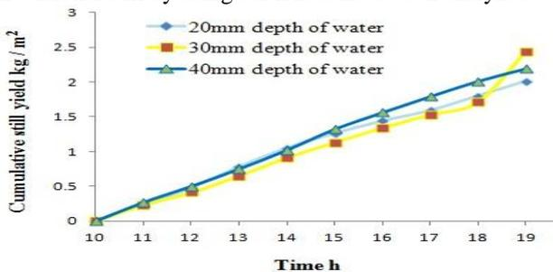
Fig. 2: Variation of still output for different depths of saline water in the modified still using earth heat without any energy storage medium
