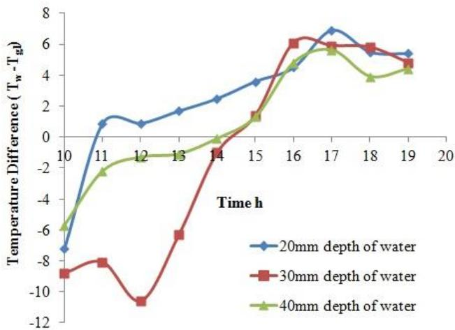
Fig. 5: Temperature differences for different depths of saline water and glass cover for the same climatic condition in the modified still using earth heat
