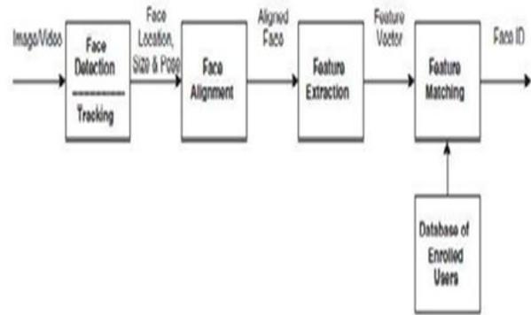
Fig. 1: Procedure for Face Recognition [6]
