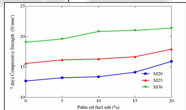
Fig. 2: 7 days Compressive strength results of concrete with palm oil fuel ash
