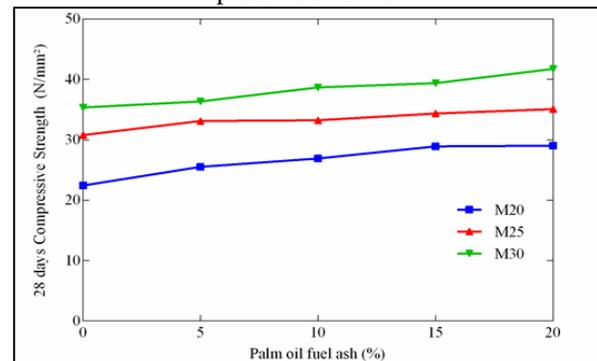
Fig. 3: 28 days compressive strength of concrete with varying amount of palm oil fuel ash
