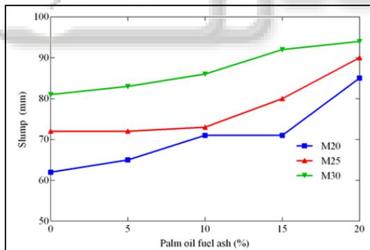
Fig. 1: Workability of concrete with varying amount of palm oil fuel ash
