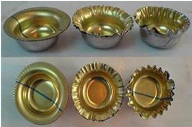
Fig. 10: The effect of decreasing the blank holder force (from left to right) on occurrence of wrinkling at the edges of composite blanks. behavior of finished part.
