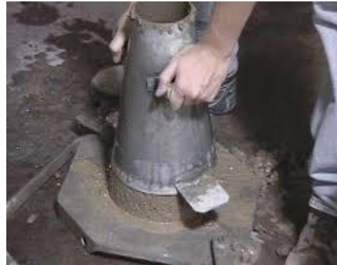
Fig. 2: Slump cone test for Workability Source: B.V.P.I.T(D.S), Umrakh
