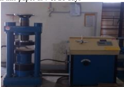
Fig. 1: Set up of Compressive Testing Machine Source: B.V.P.I.T(D.S), Umrakh
