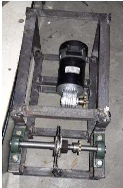
Fig. 4: Actual model of coconut de-shelling machine
