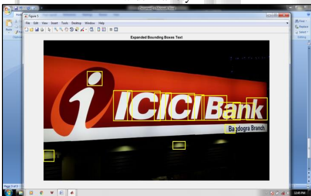
Fig. 12: Expansion of bounding boxes text
