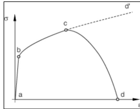
Fig. 4: Typical uniaxial stress-strain response of a metal specimen
