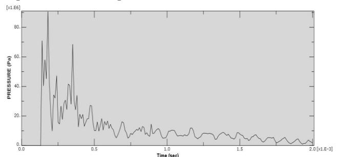
Fig. 5: Graph showing development of Hugoniot pressure due to impact of EOS bird on a rigid plate at 116m/sec
