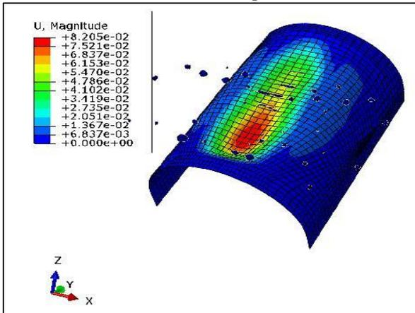
Fig. 6: Impact of 1.81 kg Bird at 150 m/sec (540 km/hr)
