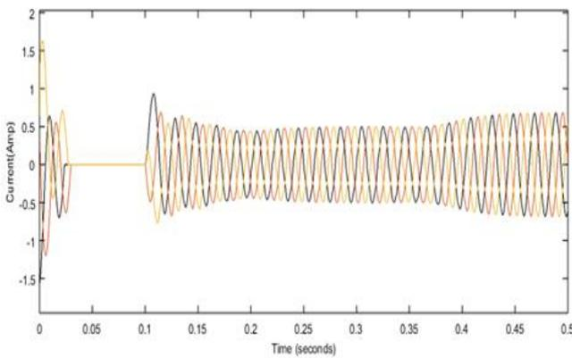
Fig. 18: Grid side current of main converter
