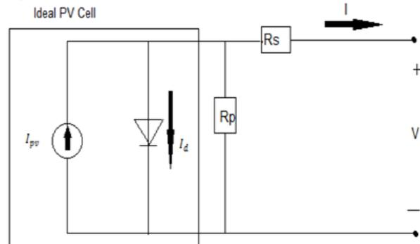
Fig. 2: PV cell single diode model
