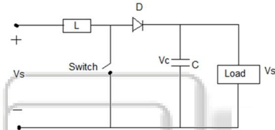
Fig. 3: Configuration of Boost converter
