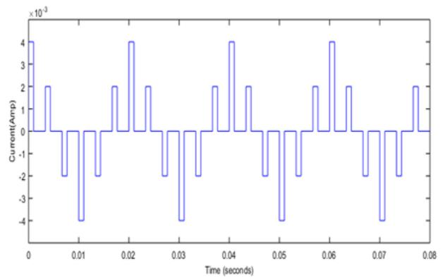
Fig. 15: Output current of main converter
