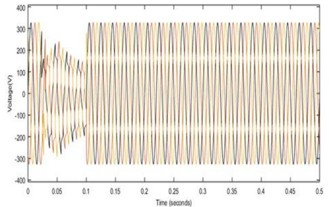
Fig. 17: Grid side voltage of main converter
