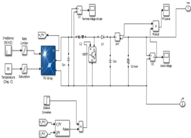
Fig. 7: Simulation of PV Array with Boost Converter
