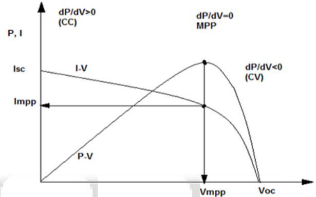
Fig. 4: PV array I-V and P-V characteristics
