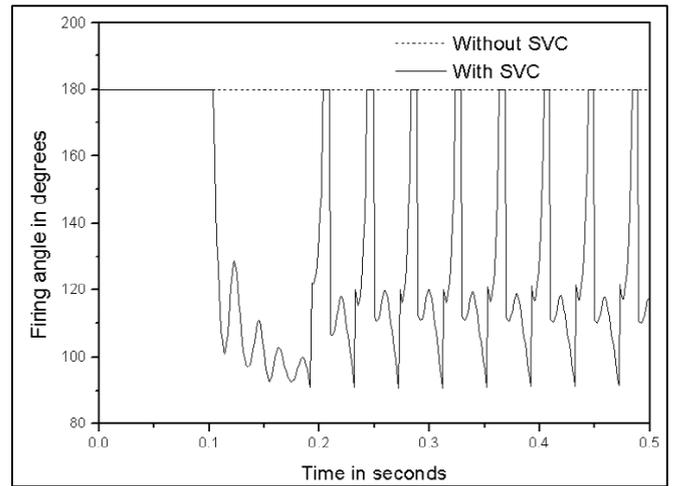
Fig. 4: The firing angle at the load with P = 4MW and Q = 3MVars
