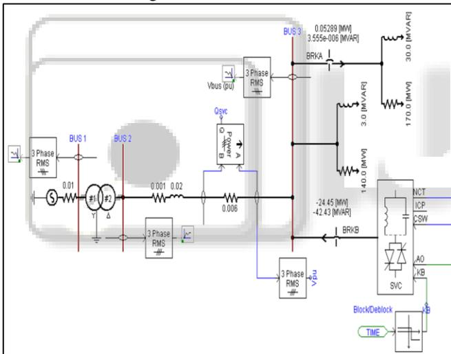
Fig. 3: a 230kV power system with SVC connected at bus3
