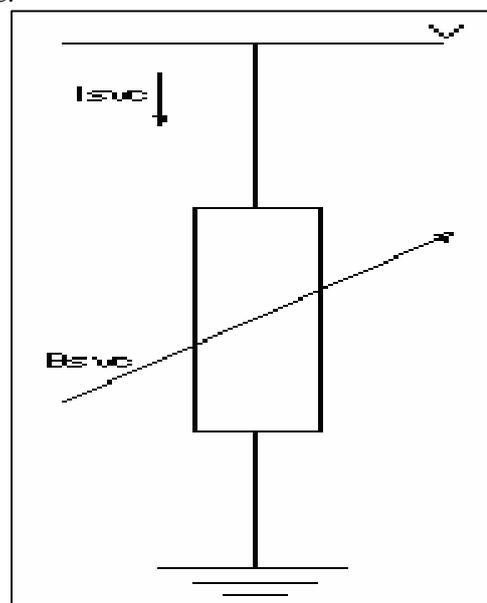
Fig. 2: Equivalent Circuit of SVC
