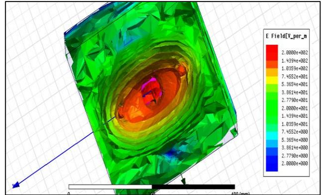
Fig. 5: The result of optimum SAR distribution for frequency value of 835 MHz at  $\phi=0$ .
