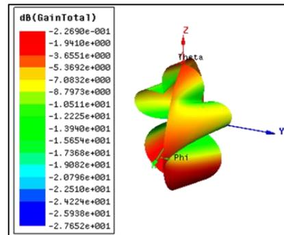
Fig. 7: Simulated 3d gain plot of the device under test  $\Phi=0$  and  $\Phi=90$  degrees at 835MHz.
