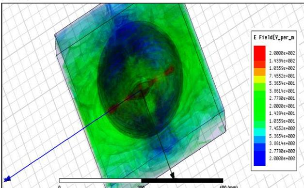
Fig. 4: SAR distribution in Brain fluid after conducting optimization for frequency value of 835 MHz at  $\phi=0$ .
