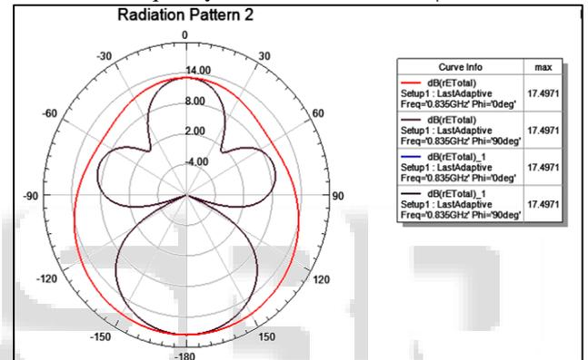
Fig. 6: Simulated radiation pattern of the dipole antenna for  $\Phi=0$  and  $\Phi=90$  degrees at 835 MHz.
