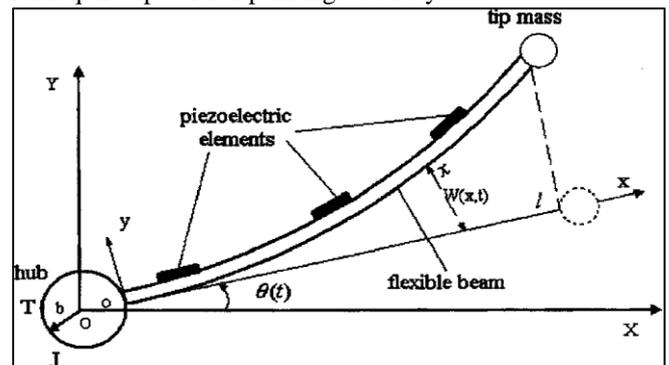
Fig. 1: Model of spacecraft with flexible appendages with bonded PZT material
