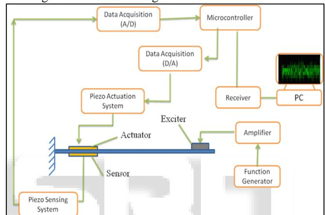
Fig. 3: Experimental setup for Active Vibration Control
