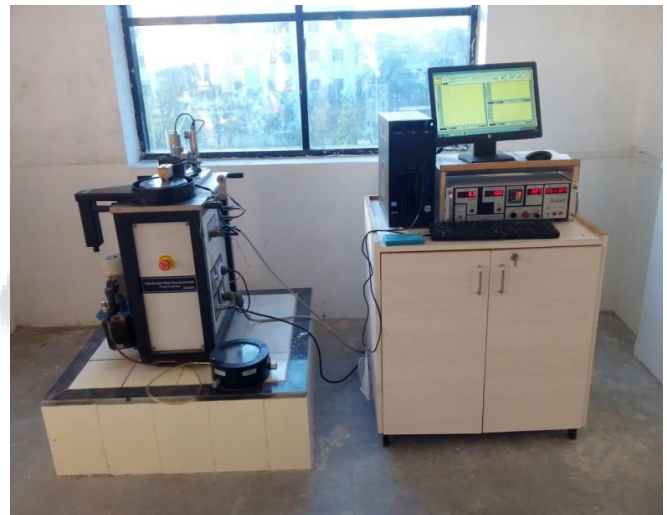
Fig. 1: Experimental Setup for Friction and Wear test (Pin on Disc Apparatus)
