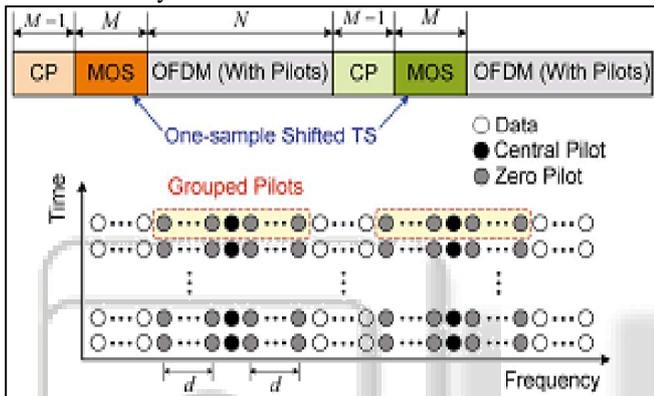
Fig. 1: Joint Time-Frequency signal structure for TDS-OFDM [1]
