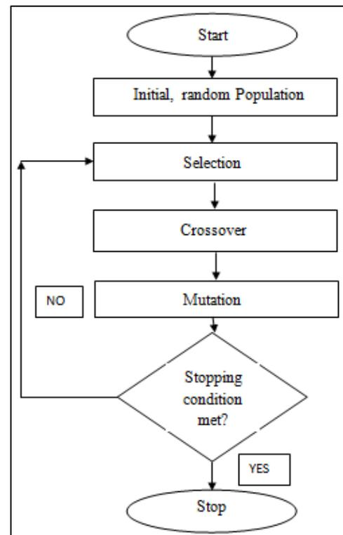
Fig. 3: Genetic Algorithm Flowchart
