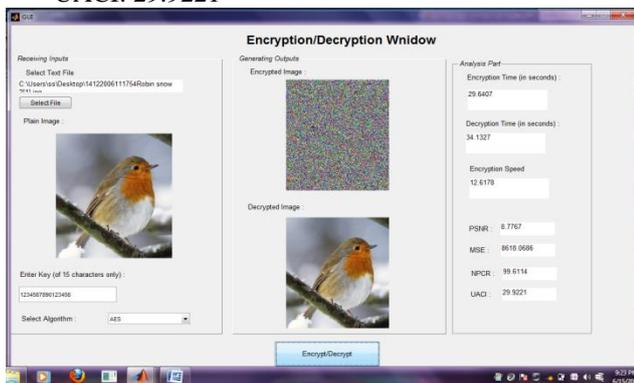
Fig. 2: Encryption of Image with AES
