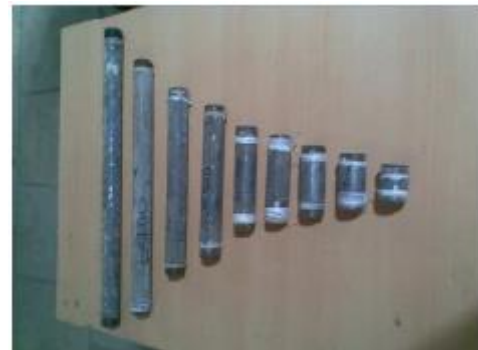
Fig. 5: Photography of Nine different upstream pipe lengths.
