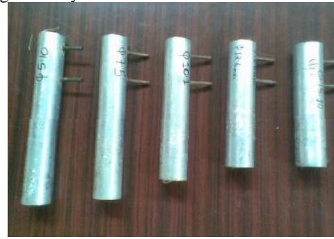
Fig. 4: Photography of Manufactured Five Different Beta Ratio Venturimeters.
