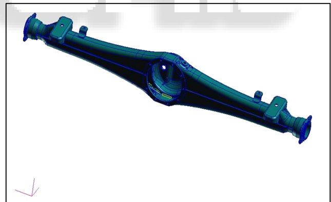
Fig. 2: CAD model of the Rear Axle Housing
