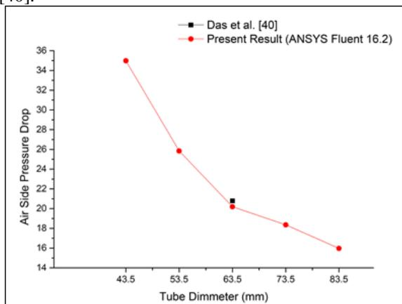
Fig. 4.11: Graph plotted between air side pressure drop and different tube diameter in Das et al. [40] and Present ANSYS Fluent 16.2 result
