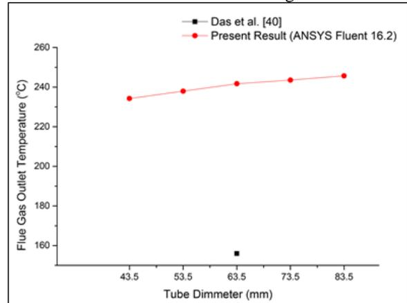
Fig. 4.8: Graph plotted between Flue gas outlet temperature and different tube diameter in Das et al. [40] and Present ANSYS Fluent 16.2 result
