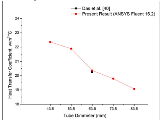
Fig. 4.12: Graph plotted between heat transfer coefficient and different tube diameter in Das et al. [40] and Present ANSYS Fluent 16.2 result
