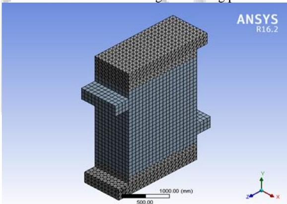
Fig. 3.1: Meshing view of Air Preheater (Isometric & Front View)
