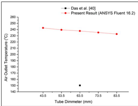
Fig. 4.9: Graph plotted between air outlet temperature and different tube diameter in Das et al. [40] and Present ANSYS Fluent 16.2 result
