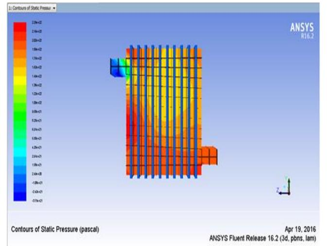
Fig. 4.2: Contour plot of static Pressure in Air Preheater (cross section) (Tube diameter 43.5)
