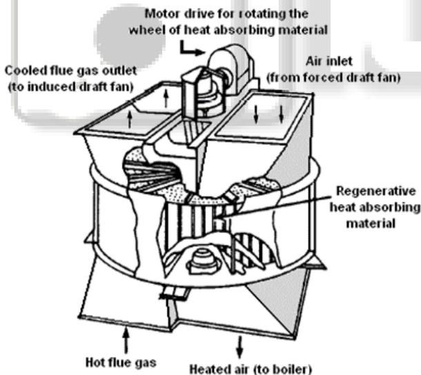
Fig. 1.3: Typical Rotating-plate Regenerative Air Preheater (Bi-sector type)
