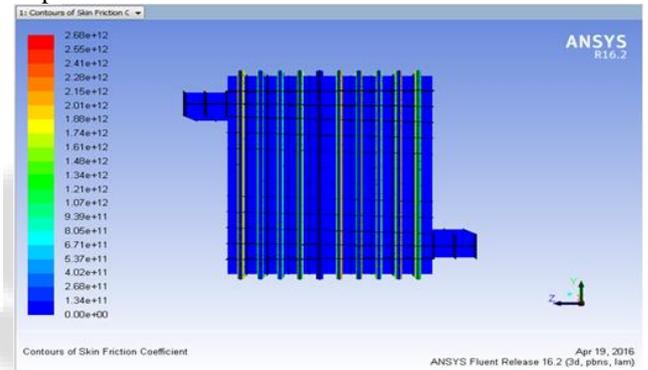
Fig. 4.7: Contour plot Skin Friction Coefficient in Air Preheater (Tube diameter 43.5)
