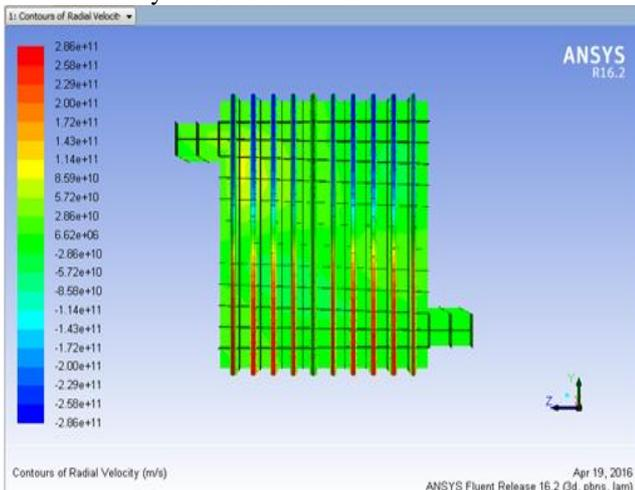
Fig. 4.5: Contour plot of Radial Velocity in Air Preheater (Tube diameter 43.5)
