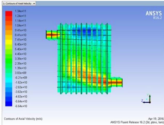
Fig. 4.4: Contour plot of Axial Velocity in Air Preheater (Tube diameter 43.5)
