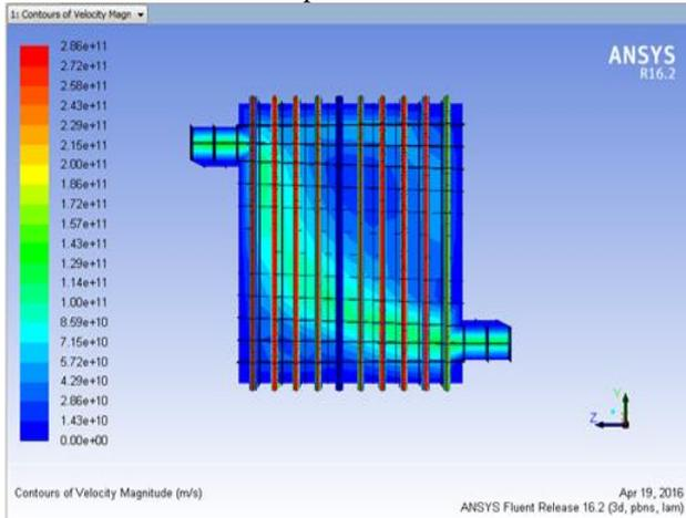
Fig. 4.3: Contour plot of Velocity magnitude in Air Preheater (cross section) (Tube diameter 43.5)
