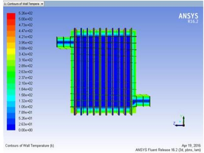
Fig. 4.6: Contour plot of wall temperature in Air Preheater (Tube diameter 43.5)
