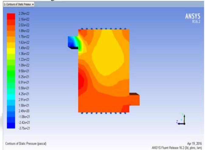
Fig. 4.1: Contour plot of Static Pressure in Air Preheater (Tube diameter 43.5)
