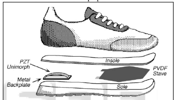
Fig. 1: Piezoelectric shoe harvester. Kymissis et al. (1998)
