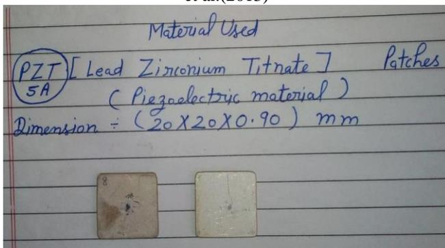
Fig. 3: Piezoelectric material used in the analysis, Varun et al.(2013)
