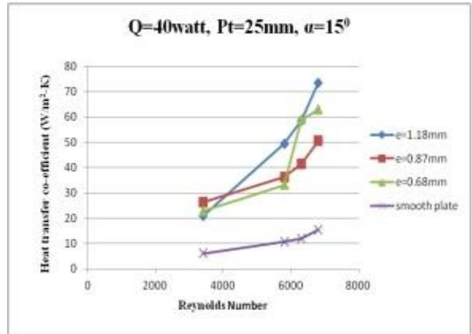
Fig. 4: shows The HTC for a constant  $\alpha=15^\circ$ ,  $Pt=25mm$  and power input (Q) =40watts and for also various Reynolds number (Re) and roughness height (e)
