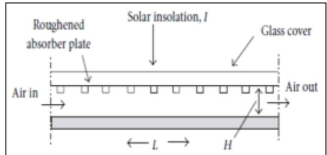
Fig. 1: typical solar air heater with extended surface
