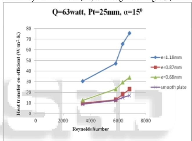
Fig. 5: shows The HTC for a constant  $\alpha=15^\circ$ ,  $Pt=25mm$  and power input (Q) =63watts and for also various Reynolds number (Re) and roughness height (e).
