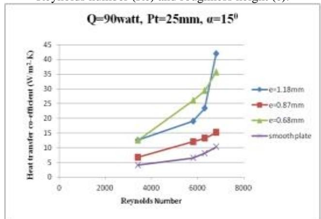
Fig. 6: shows The HTC for a constant  $\alpha=15^\circ$ ,  $Pt=25mm$  and power input (Q) =90watts and for also various Reynolds number (Re) and roughness height (e).
