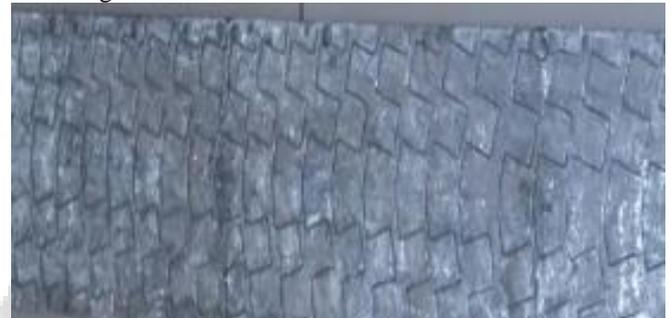
Fig. 3: aluminum absorber plate with roughness
