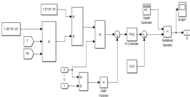
Fig. 4: Simulink model of MPPT
