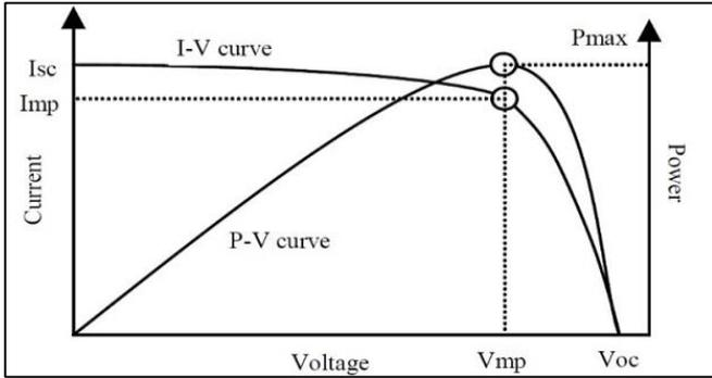
Fig. 3: I-V and PV characteristics of solar cell
