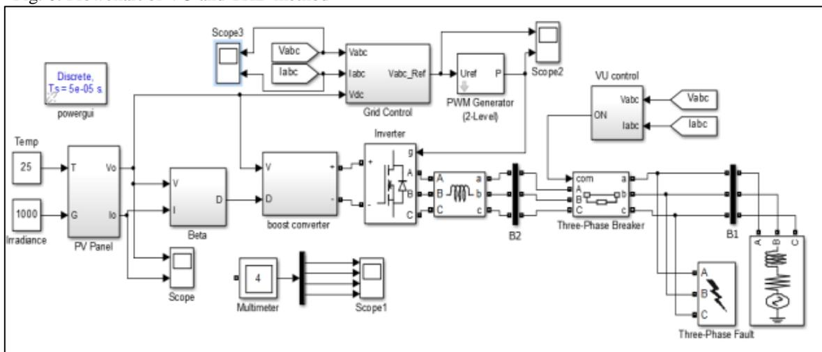
Fig. 7: Simulation model of entire system
