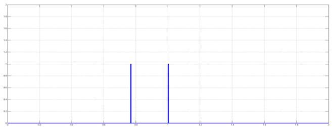
Fig. 12: Final output pulse to initiate circuit breaker (x axis: 0.2s/div, y axis: 0.5V/div)
