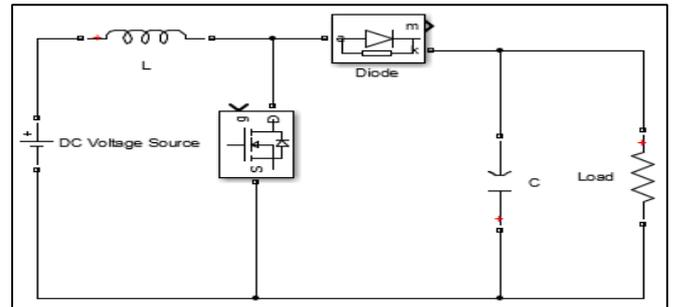
Fig. 5: Schematic diagram of boost converter
