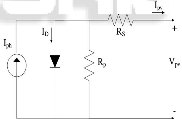
Fig. 2: Single diode equivalent circuit of PV cell
