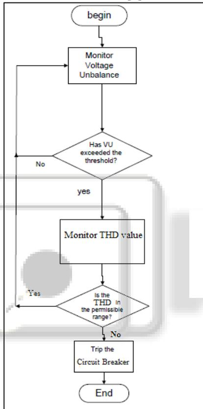
Fig. 6: Flowchart of VU and THD method
