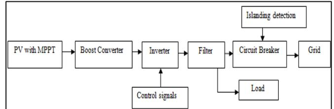
Fig. 1: Block Diagram of DG interfaced Grid system
