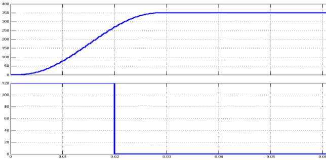
Fig. 9: Output voltage waveform of boost converter with (x axis: 0.01s/div, y axis: 50V/div)
