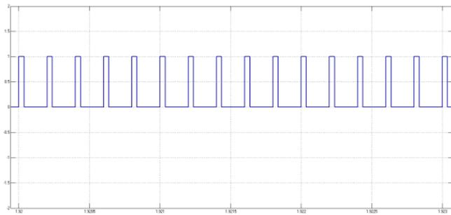
Fig. 8: Pulses to the switch of boost converter (x axis: 0.05 ms/div, y axis: 0.5V/div)
