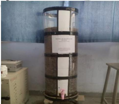
Fig. 9: Model of Rapid Sand Filter Filled With Material
