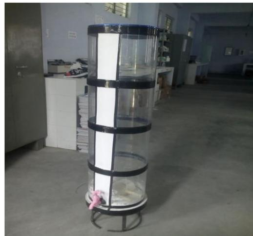
Fig. 3: Model of Rapid Sand Filter
