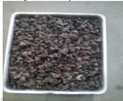
Fig. 4: Coarse Gravel 20mm size
