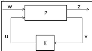
Fig. 2: Block Diagram of H-infinity Controller.
