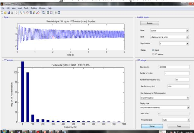
Fig. 5: THD of three phase inverter with H-infinity controller
