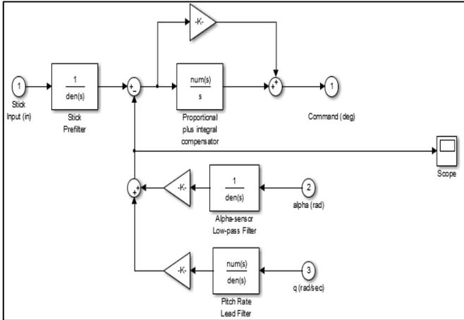
Fig. 3: MATLAB model of H-infinity controller
