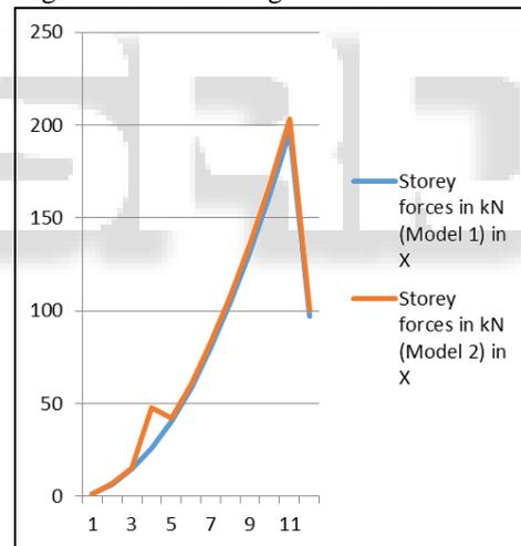
Fig. 26: Storey vs. Storey forces in X (kN)
