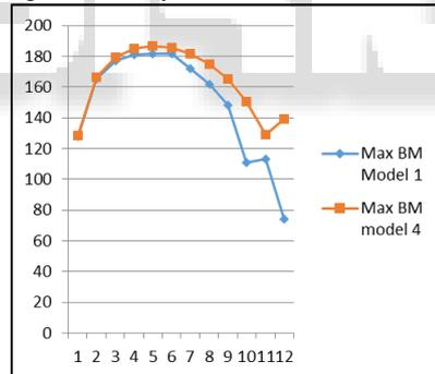
Fig. 13: Storey vs. Max BM in( kN-m)
