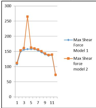
Fig. 7: Storey vs. Max SF(in kN)
