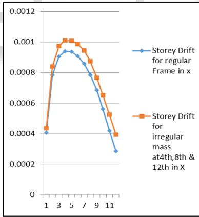
Fig. 21: Storey vs. Storey Drift in X (m)
