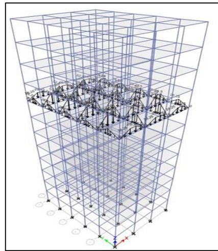
Fig. 4: 3D view of Frame with lumped mass at 8th floor
