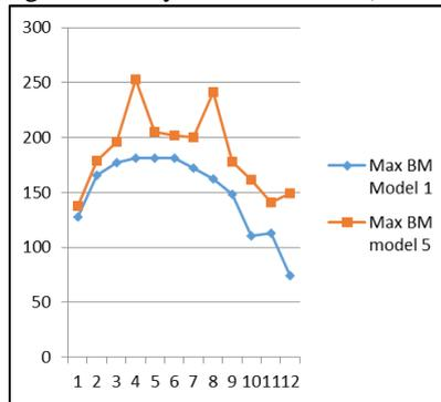
Fig. 14: Storey vs. Max BM in( kN-m)
