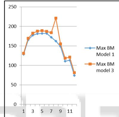
Fig. 12: Storey vs. Max BM (in kN-m)
