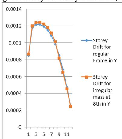
Fig. 18: Storey vs. Storey Drift in Y (m)
