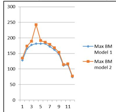
Fig. 11: Storey vs. Max BM(in kN-m)
