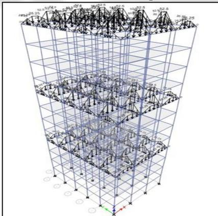
Fig. 6: 3D view of Frame with lumped mass at 4<sup>th</sup>, 8<sup>th</sup> & 12<sup>th</sup> floor
