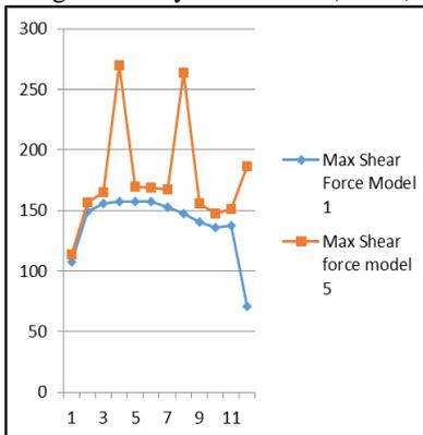
Fig. 10: Storey vs. Max SF(in kN)
