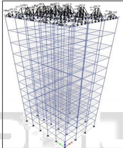
Fig. 5: 3D view of Frame with lumped mass at 12th floor
