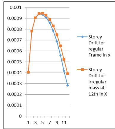
Fig. 19: Storey vs. Storey Drift in X ( m)
