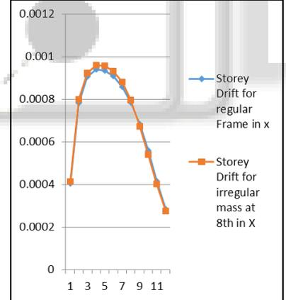
Fig. 17: Storey vs. Storey Drift in X ( m)
