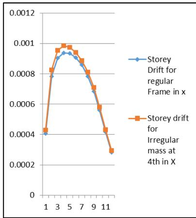
Fig. 15: Storey vs. Storey Drift in X ( m)
