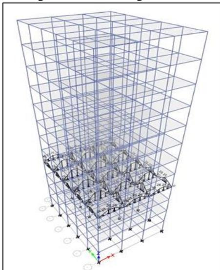
Fig. 3: 3D view of Frame with lumped mass at 4th floor
