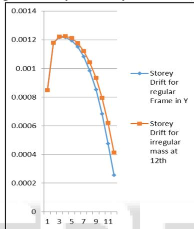
Fig. 20: Storey vs. Storey Drift in Y ( m)
