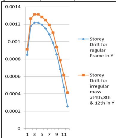
Fig. 22: Storey vs. Storey Drift in Y (m)
