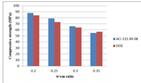
Fig. 1: Comparison of compressive strength for mix proportioning of high strength concrete with angular aggregate
