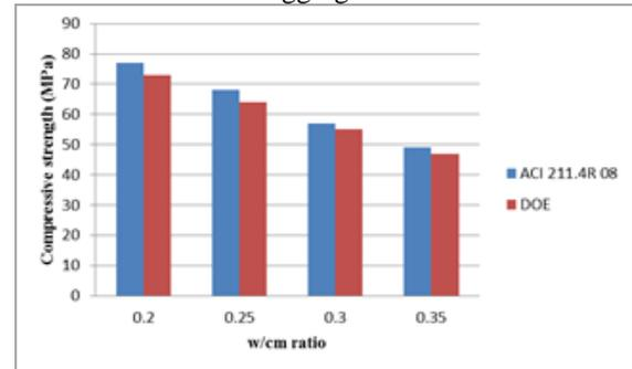
Fig. 2: Comparison of compressive strength for mix proportioning of high strength concrete with angular aggregate
