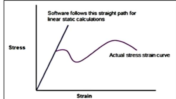
Fig. 4: Linear Static Approach
