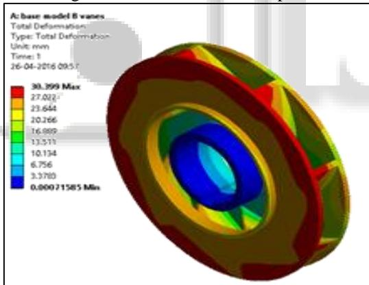
Fig. 6: Total deformation of impeller pump
