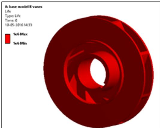
Fig. 6: Life evaluation of impeller
