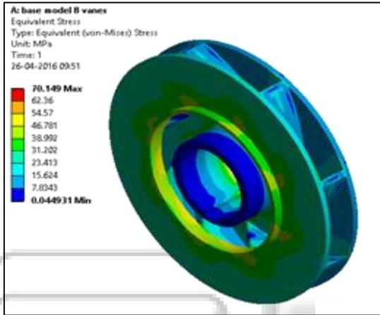
Fig. 5: Von-mises stress of impeller
