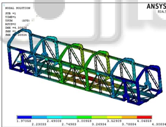
Fig. 6: Deformation due to self-weight of traverser before optimization (4.308 mm)
