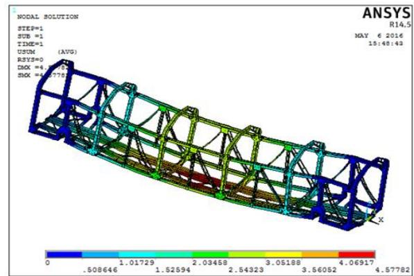
Fig. 8: Deformation due to self-weight after topology optimization (4.577 mm)
