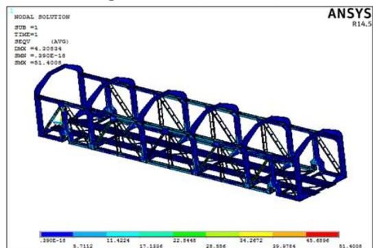
Fig. 7: Vonmises Stress due to self-weight before optimization (51.008 Mpa)
