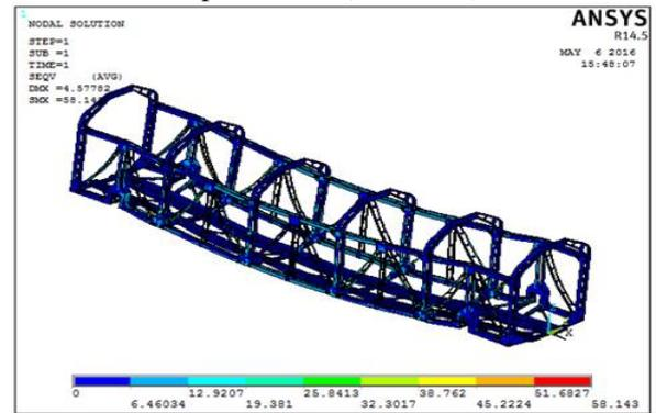
Fig. 9: Vonmises stress due to self-weight after topology optimization (58.143 Mpa)
