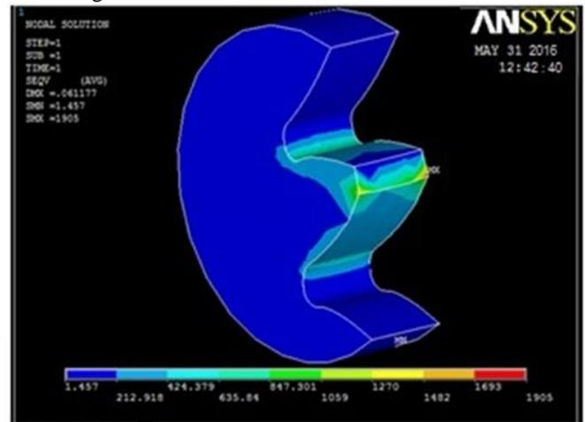
Fig. 4: Von-Misses Stress Distribution of asymmetric gear.
