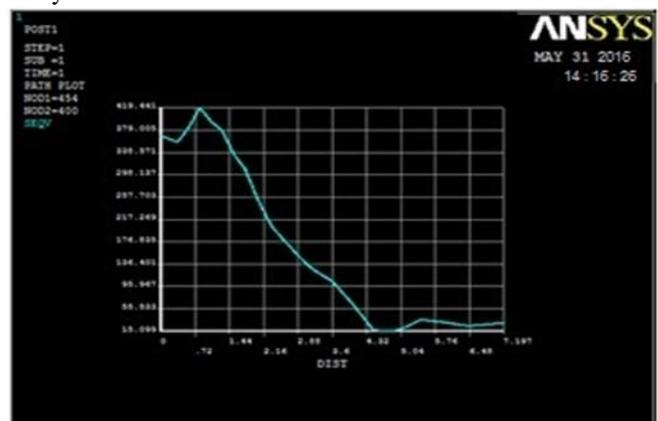
Fig. 8: Graph of Von-Misses Stress Distribution at fillet area of asymmetric gear with hole at third trial.
