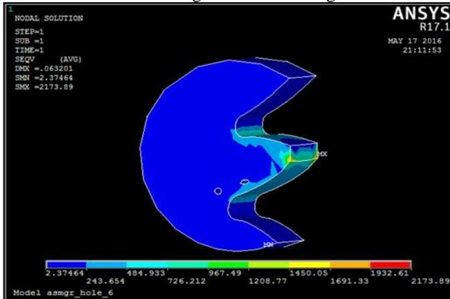
Fig. 15: Contour Plot of Von-Misses Stress Distribution at fillet area of asymmetric gear with composite holes as stress relieving feature as per Modification-2.
