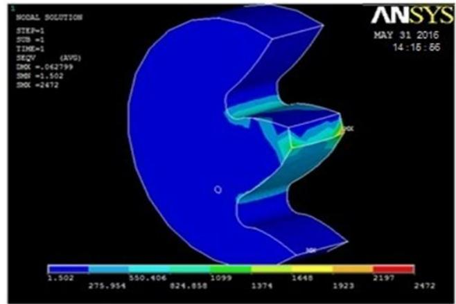
Fig. 7: Contour plotting of stress on whole the gear tooth and near hole.
