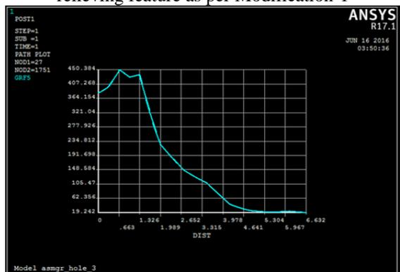
Fig. 14: Graph of Von-Misses Stress Distribution at fillet area of asymmetric gear with composite holes as stress relieving feature as per Modification-1
