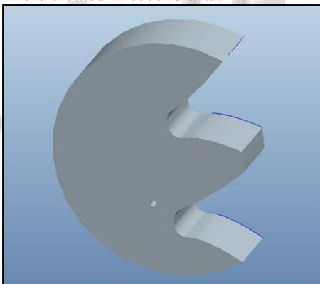
Fig. 6: Isometric view of 3-D asymmetric gear with hole in 3rd trial
