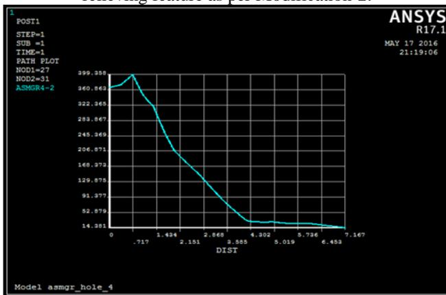
Fig. 16: Graph of Von-Misses Stress Distribution at fillet area of asymmetric gear with composite holes as stress relieving feature as per Modification-2
