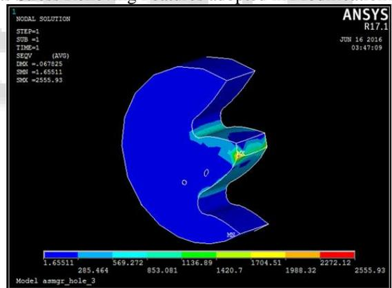
Fig. 13: Contour Plot of Von-Misses Stress Distribution at fillet area of asymmetric gear with composite holes as stress relieving feature as per Modification-1
