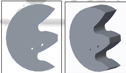
Fig. 12: A & B: Front view and isometric view of asymmetric gear with composite holes as stress relieving feature as per Modification-1
