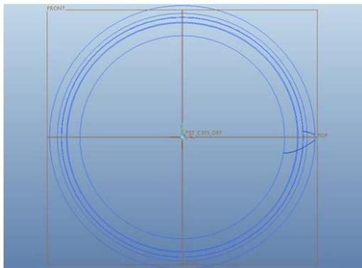
Fig. 1: Involute curves for asymmetric gear.
