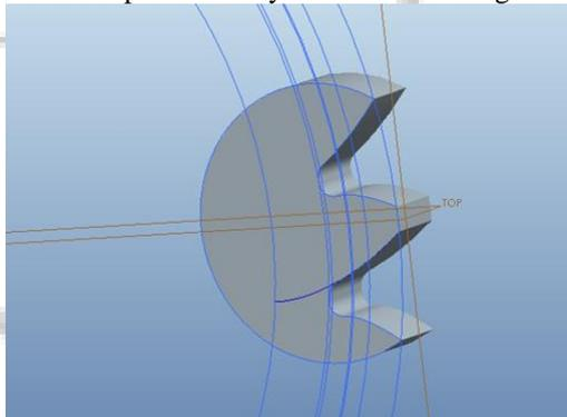
Fig. 3: 3-Dimensional model of an asymmetric gear tooth
