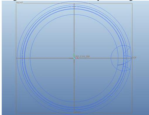
Fig. 2: Partial profile of asymmetric involute gear tooth.
