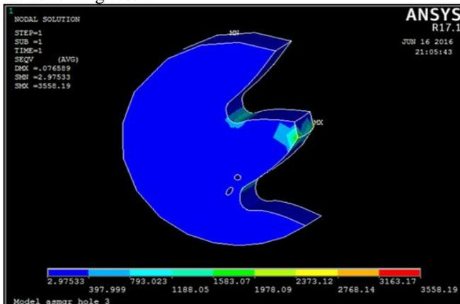
Fig. 17: Contour Plot of Von-Misses Stress Distribution at fillet area of asymmetric gear with composite holes as stress relieving feature as per Modification-3
