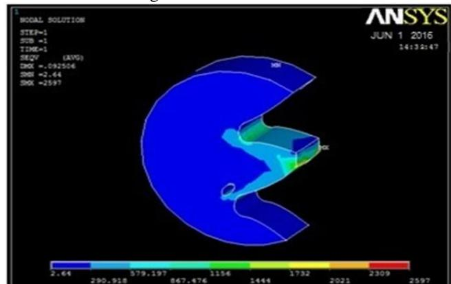
Fig. 10: Contour plotting of stress on whole the gear tooth and near hole.
