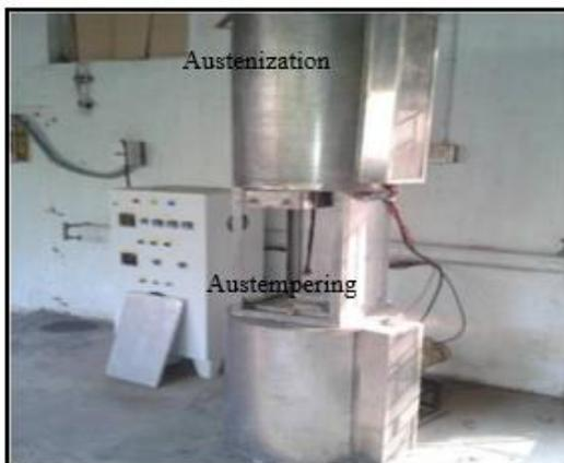
Fig. 4: Austempering Furnace
