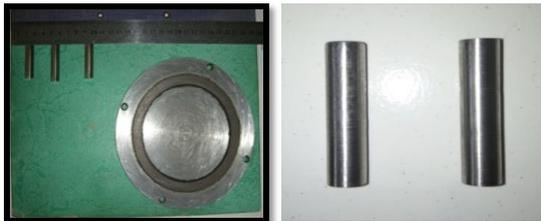
Fig. 15: The Diamond Coated Disc and Samples of CADI
