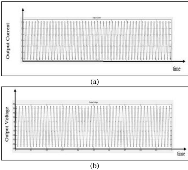
Fig. 14: Output current (a) and output voltage (b) waveforms of Buck-Boost AC-AC Converter
