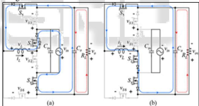
Fig. 4: Buck operation during negative cycle. (a) during DT interval (b) during 1-D interval
