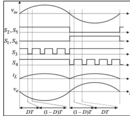
Fig. 8: Operation and key waveforms of inverting buck boost mode
