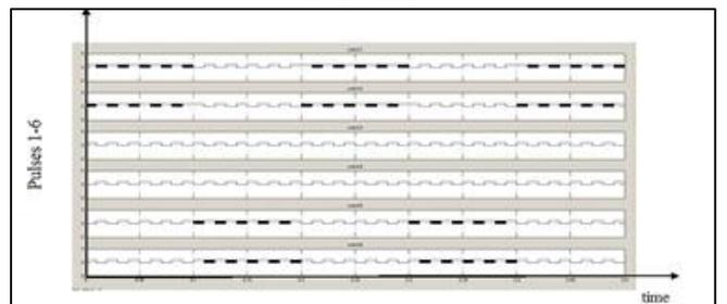
Fig. 13: Gating pulses for switches from  $S_1$  to  $S_6$  of the Buck-Boost AC-AC Converter
