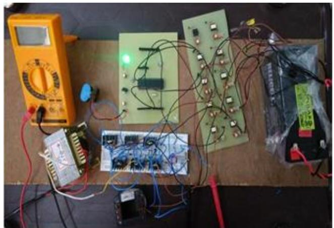
Fig. 16: Experimental setup of AC-AC Buck Boost Converter
