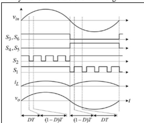
Fig. 2: Operation and key waveforms of noninverting buck mode
