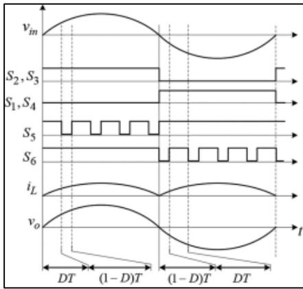
Fig. 5: Operation and key waveforms of noninverting boost mode
