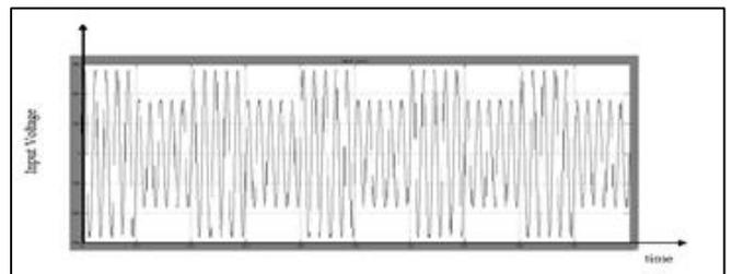
Fig. 12: Input voltage waveform of the Buck-Boost AC-AC Converter
