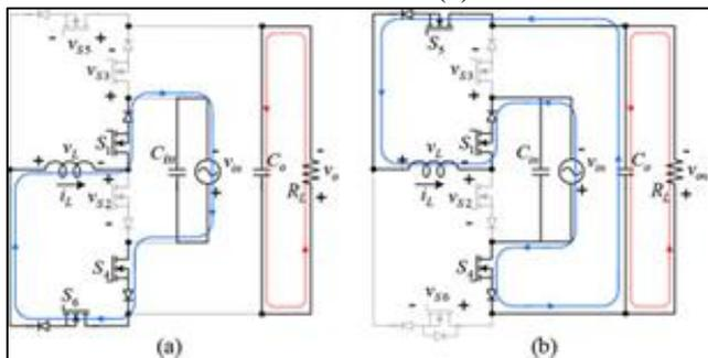
Fig. 7: Boost operation during negative cycle. (a) during  $DT$  interval (b) during  $1-D$  interval
