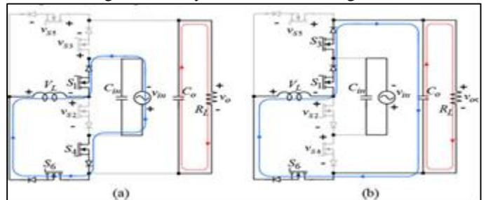
Fig. 10: Buck Boost operation during negative cycle. (a) during  $DT$  interval (b) during  $1-D$  interval
