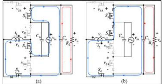
Fig. 3: Buck operation during positive cycle. (a) during DT interval (b) during 1-D interval
