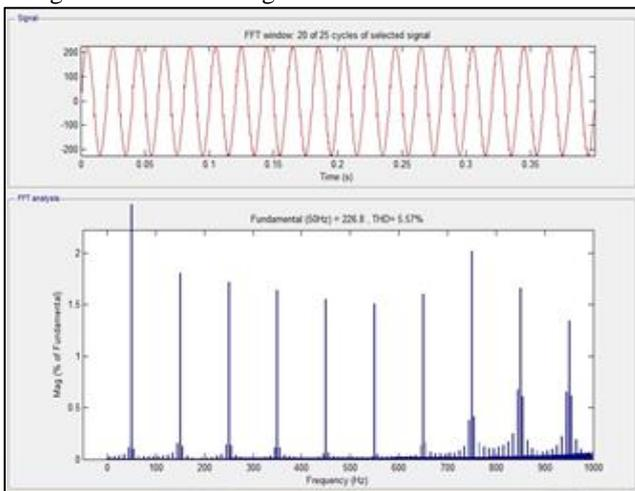
Fig. 15: THD of output voltage waveform
