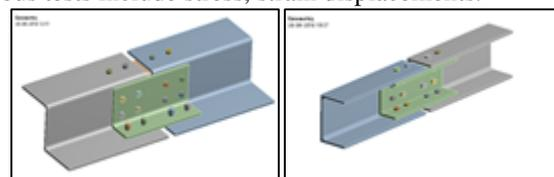
Fig. 2: Isometric view of L-type and U- type splice joint
