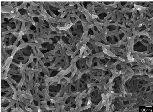
Fig. 2: SEM images of Polyaniline Nanofiber (PANI) 100nm
