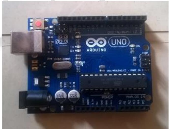
Fig. 4: Arduino Uno circuit used with the soil moisture sensor
