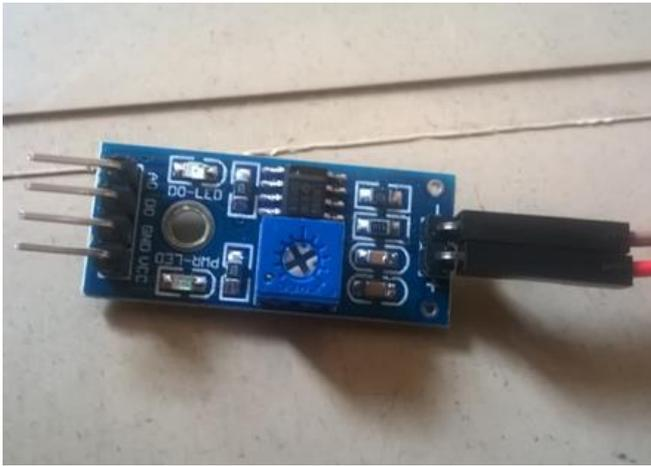
Fig. 5: LM393 used between the sensor and Arduino circuit to provide stable outputs to the microcontroller
