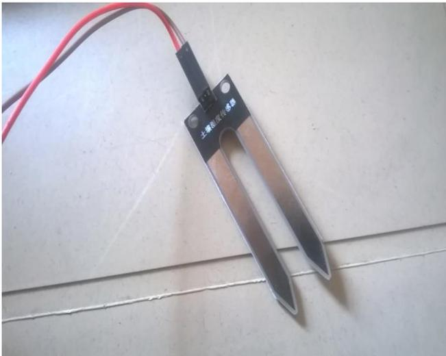
Fig. 1: YL-69 sensor used for this work
