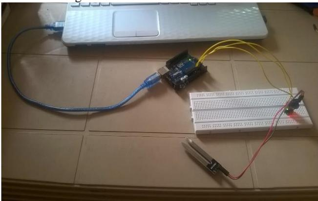
Fig. 6: Experimental setup used for the soil moisture sensing in this work
