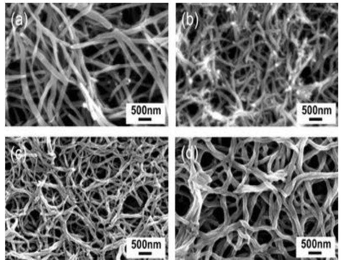
Fig. 3: SEM images of Polyaniline Nanofiber (PANI) 500nm
