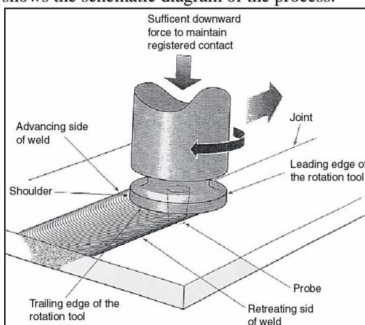
Fig. 1: Schematic of FSW [2]
