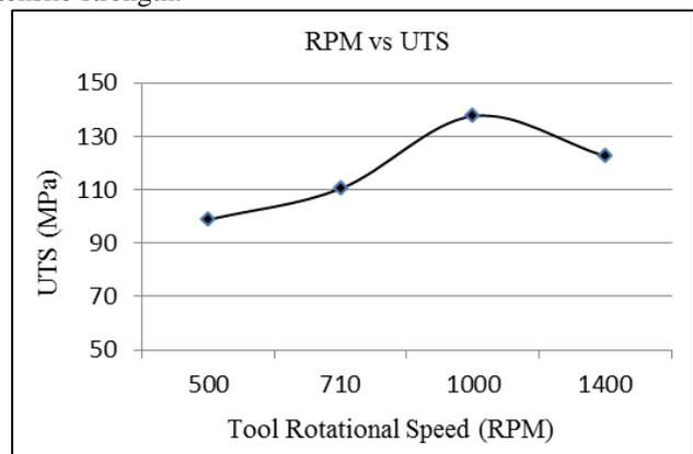
Fig. 5: Effect of Tool Rotational Speed
