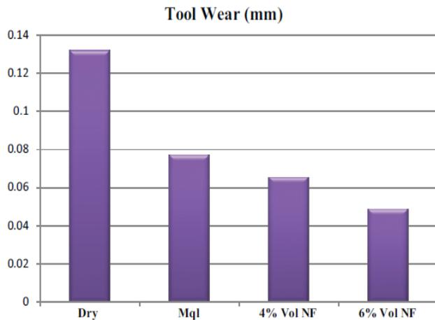
Fig. 5: Tool Wear Verses Different Cutting Conditions[6]
