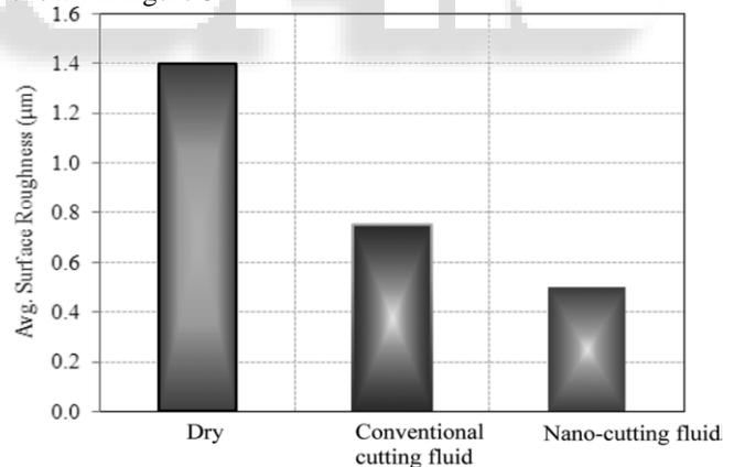
Fig. 4: Variation of Average surface roughness while dry machining and machining with conventional and nano-cutting fluid[13]
