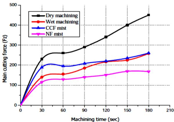
Fig. 2: Main Cutting Force versus machining time [9]
