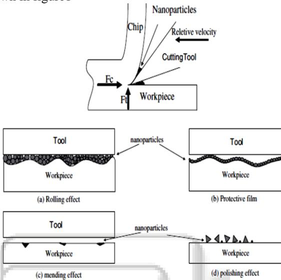
Fig. 1: Mechanism of Nanoparticle Functioning [11]
