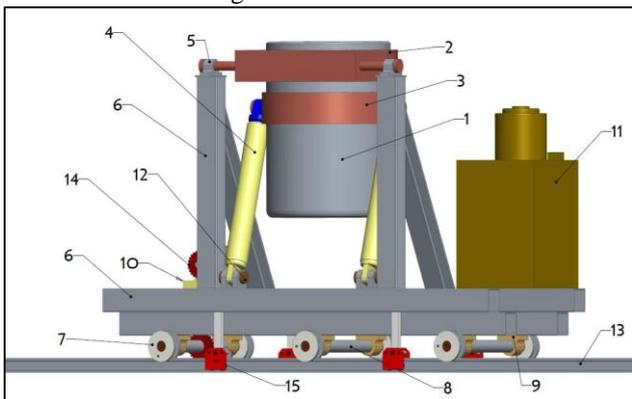
Fig. 1: Automated Ladle Transport Vehicle (ALTV)
