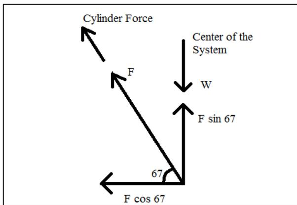
Fig. 7: Weight balancing
