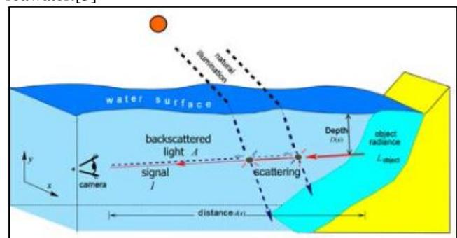
Fig. 1: Underwater optical imaging model.
