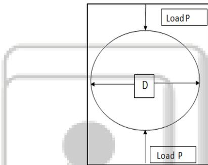
Fig. 1: Circular Disc under Diametral Compression
