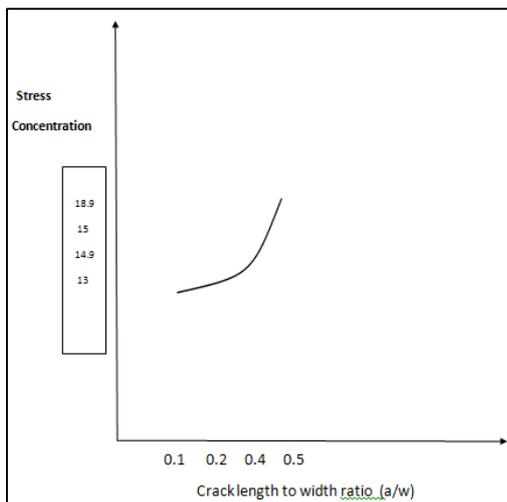
Fig. 4: The graph is plotted between stress concentration factor & crack length to width ratio
