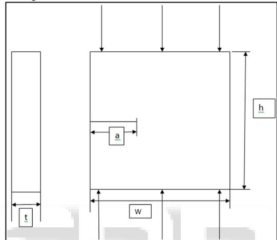
Fig. 2: Plate with an edge crack
