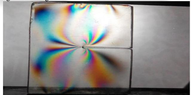
Fig. 3: Fringes of epoxy resin plate
