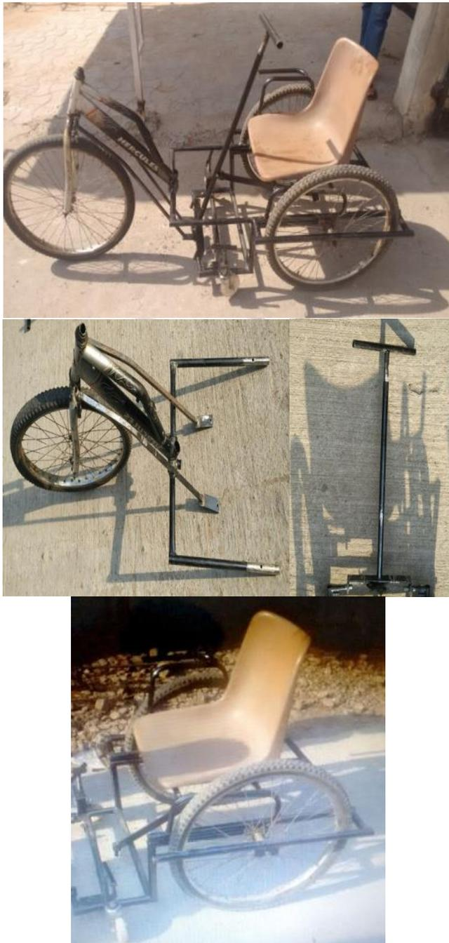
Fig. 2: Fabricated Prototype of Wheelchair cum Tricycle with Disassembly.
